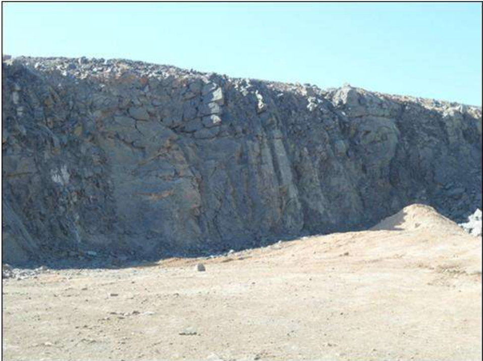
Figure 8-3 Blocky magnetite seam conditions, Vametco
