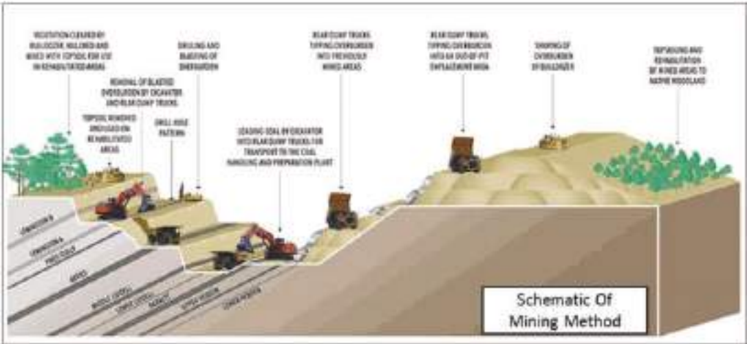
Fig 7: Schematic of the Mining Method at Vametco Mine
