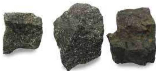
Figure 3a: Samples of massive (right), heavily disseminated (middle) and lightly disseminated (left) ore, typical of the lower vanadium-bearing magnetite at the Brits Vanadium Project
