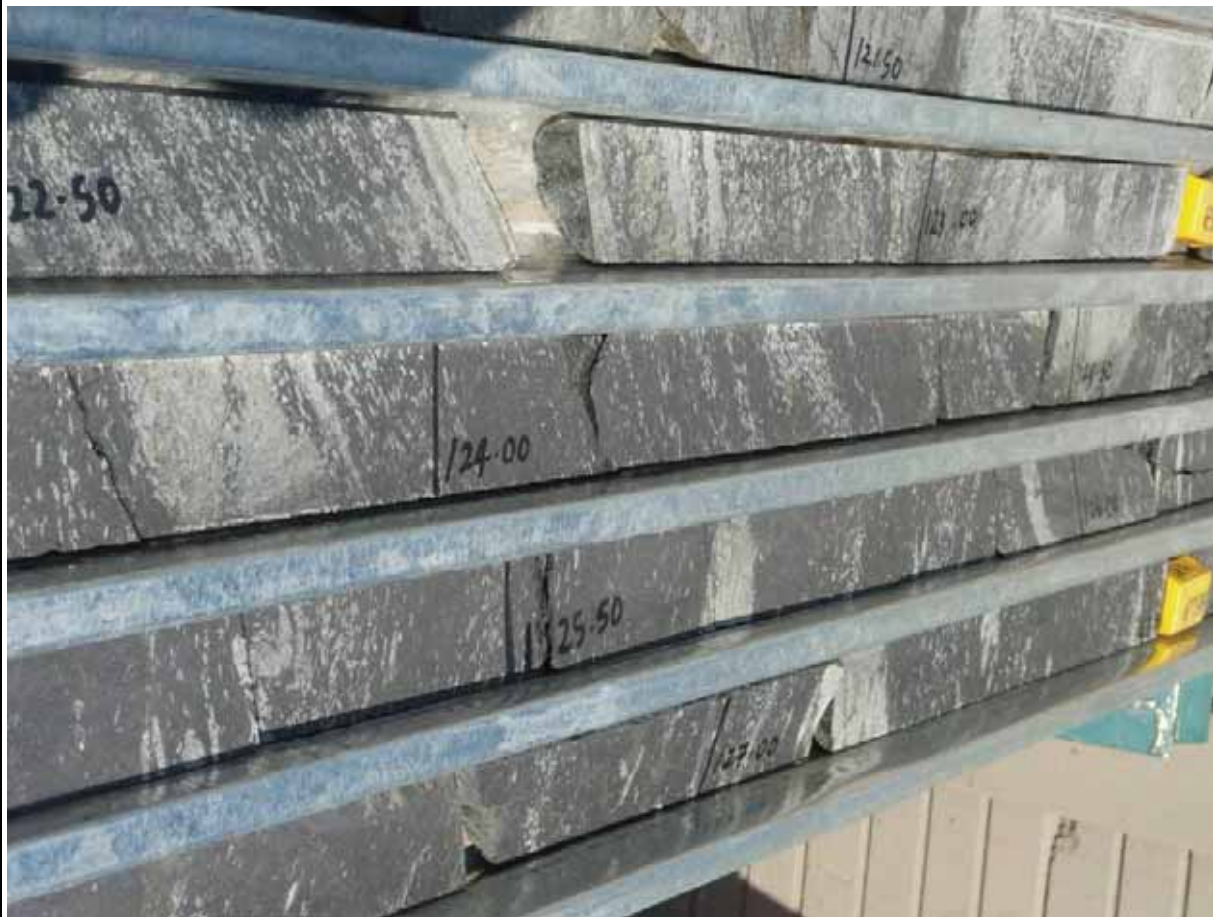
Figure 7-15 Close-up of VTM-rich and VTM-poor banding in the Q Layer of VK2
