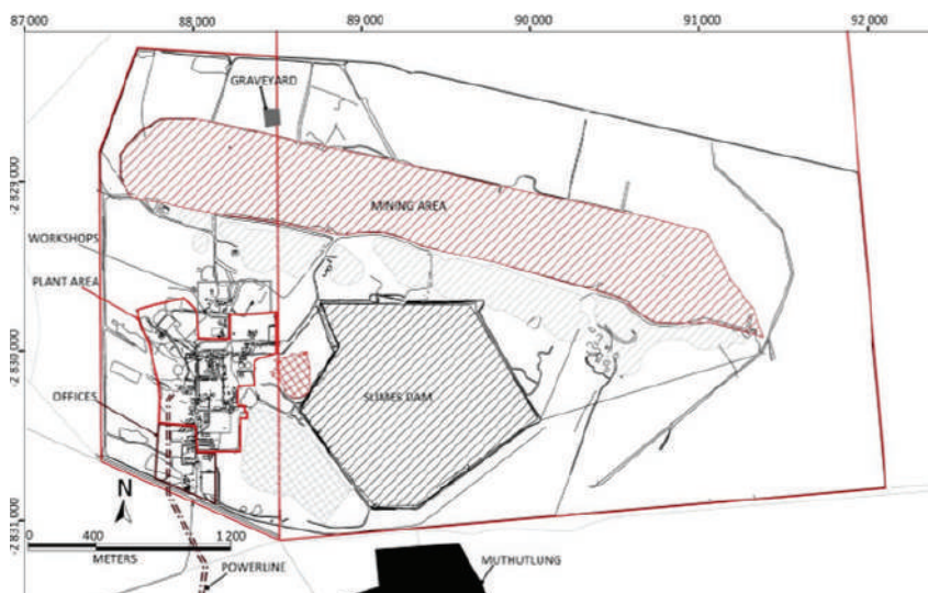
Fig 6: Layout of Infrastructure within Mining Area
