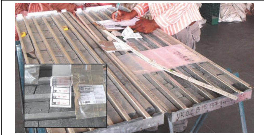
Figure 11-3 Sampling utensils; ticket book and Certified Reference Material (CRM) in inset (BML, 2011)
